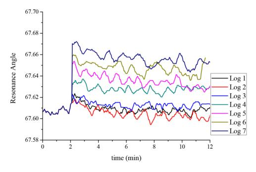
Figure 7. The trend of the measured resonance angle for each concentration of E. coli with Type 2 injection. Increasing the bacterial concentration increases the resonance angle.
