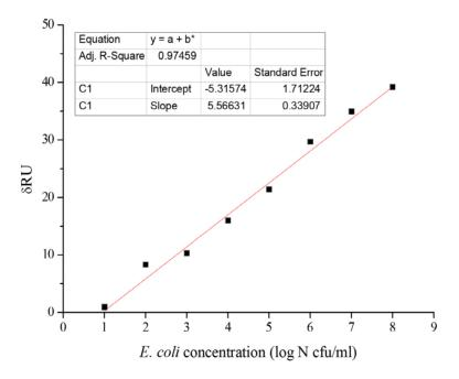
Figure 4. The lineer relationship between the change in the response unit and concentrations of Escherichia coli.
