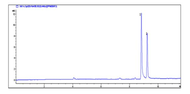
**Figure 3.** Representative electropherogram obtained from tablet dosage forms Lustral<sup>®</sup> under optimum conditions, at 205 nm absorbance, (1) SER and (2) CIT (IS).
