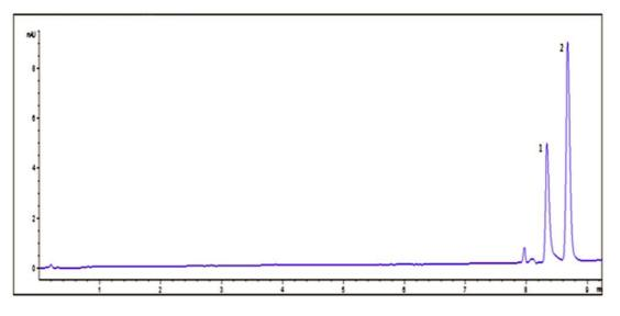
Figure 2. The electropherogram of standard (1) SER and (2) CIT (IS) under optimum conditions.
