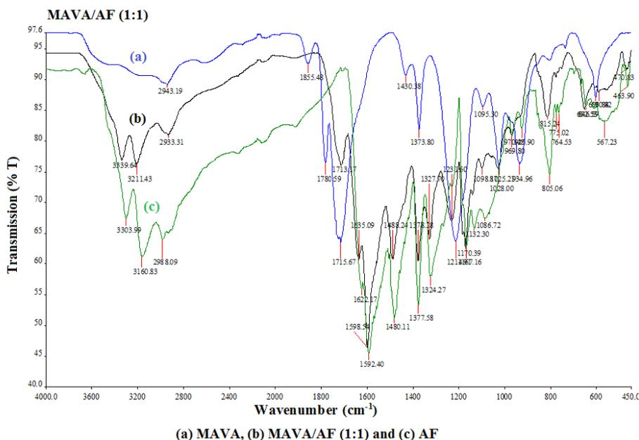
**Figure 2.** Overlapped FTIR spectra of the copolymer, conjugate and AF. (a) MAVA, (b) MAVA/AF (1:1), and (c) AF.
