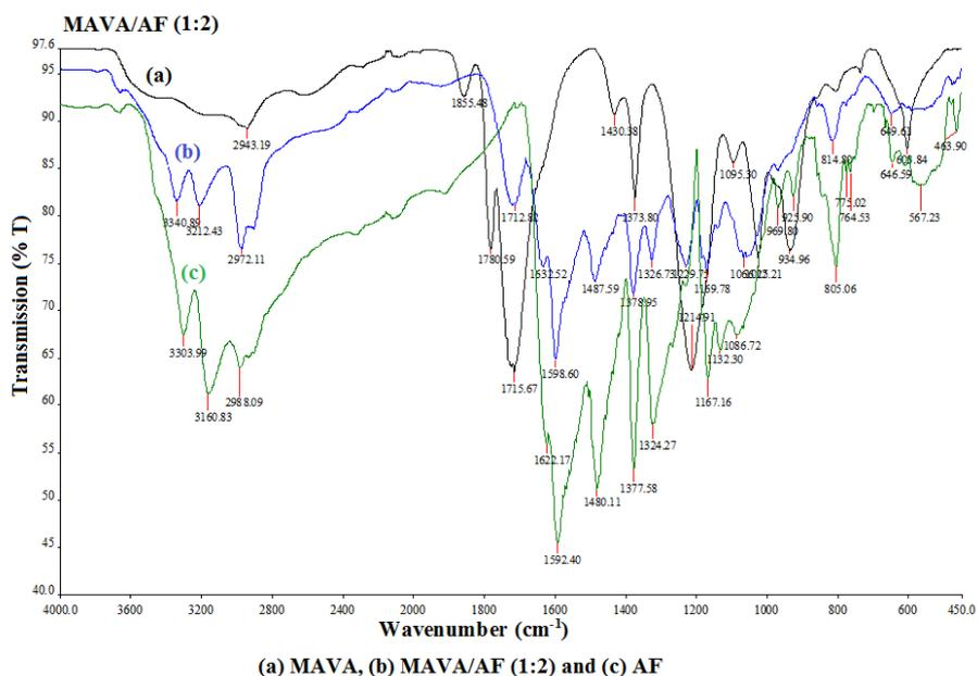
**Figure 3.** Overlapped FTIR spectra of the copolymer, conjugate and AF. (a) MAVA, (b) MAVA/AF (1:2), and (c) AF.
