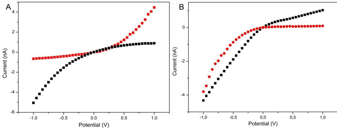
**Figure 4.** Current-voltage curves taken in 10 mM KCl, 10 mM PBS buffer before and after modification with insulin at pH 4 (A), pH 8 (B). (Before modification = black, After modification = red).
