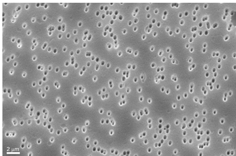
**Figure 2.** SEM images of chemically etched multipore PET membrane surface.
