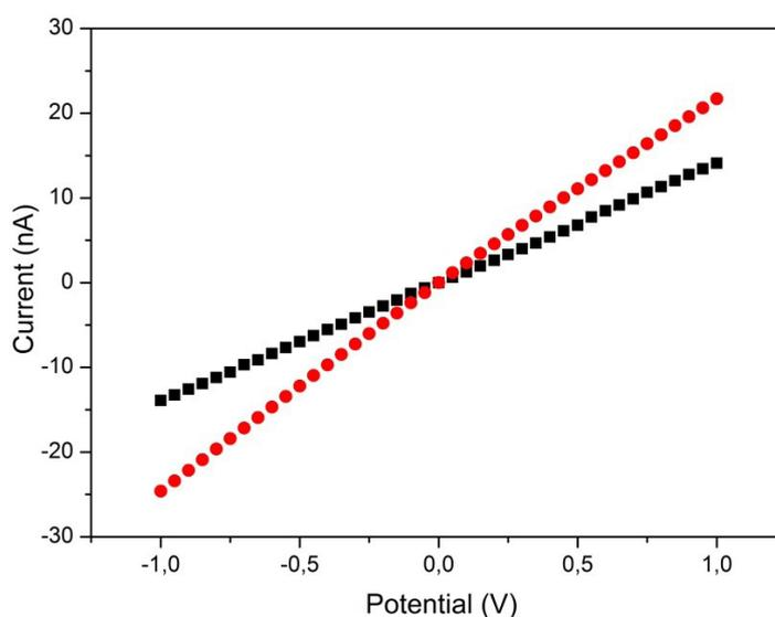
**Figure 3.** Current-voltage curves taken in 1 M KCl before and after modification to measure the change in tip diameter (black ■:  $d \sim 22$  nm), after modification with insulin (red ●:  $d \sim 17$  nm).
