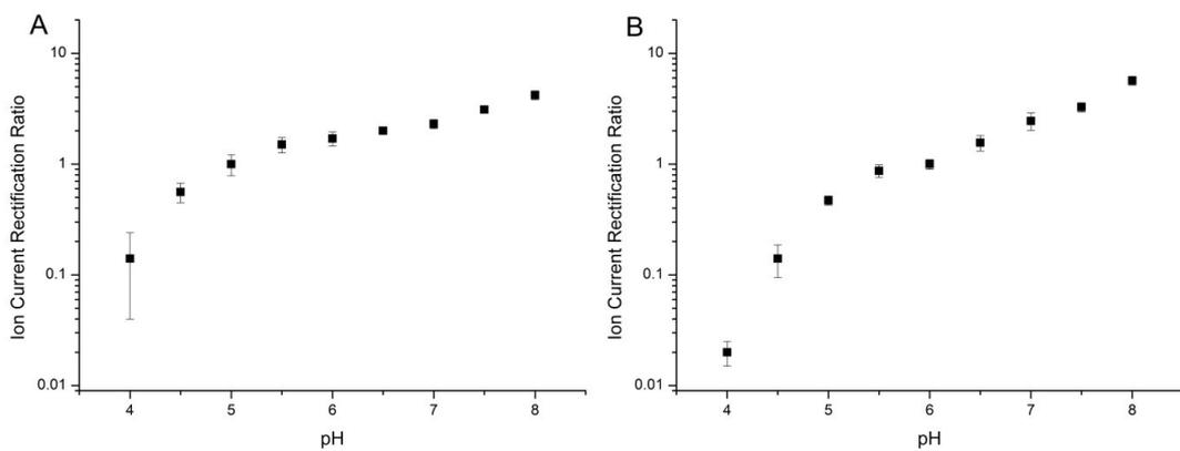
**Figure 6.** Plot of Ion-current rectification versus pH of Insulin (A), Bovine Hemoglobin (B).
