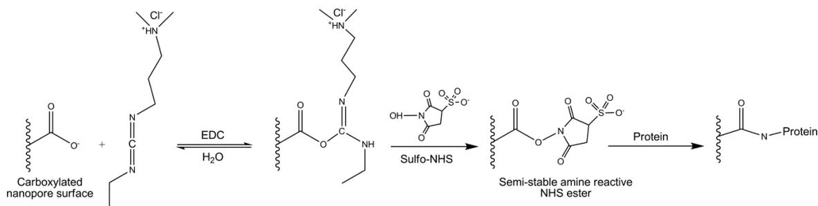
**Figure 1.** Reaction scheme for the attachment of protein to the carboxylated nanopore surface.
