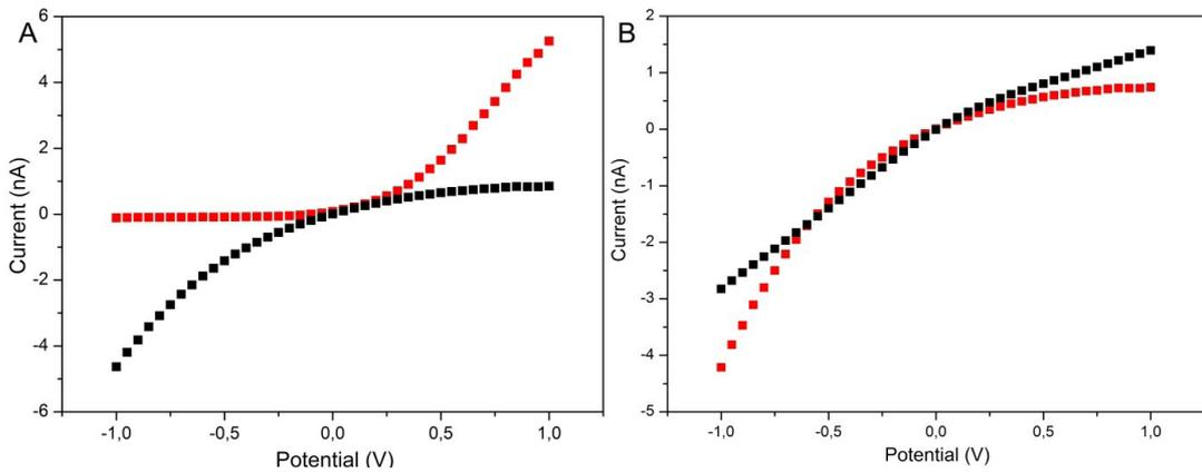
**Figure 5.** Current-voltage curves taken in 10 mM KCl, 10 mM PBS buffer before and after modification with bovine hemoglobin at pH 4 (A), pH 8 (B). (Before modification = black, After modification = red).
