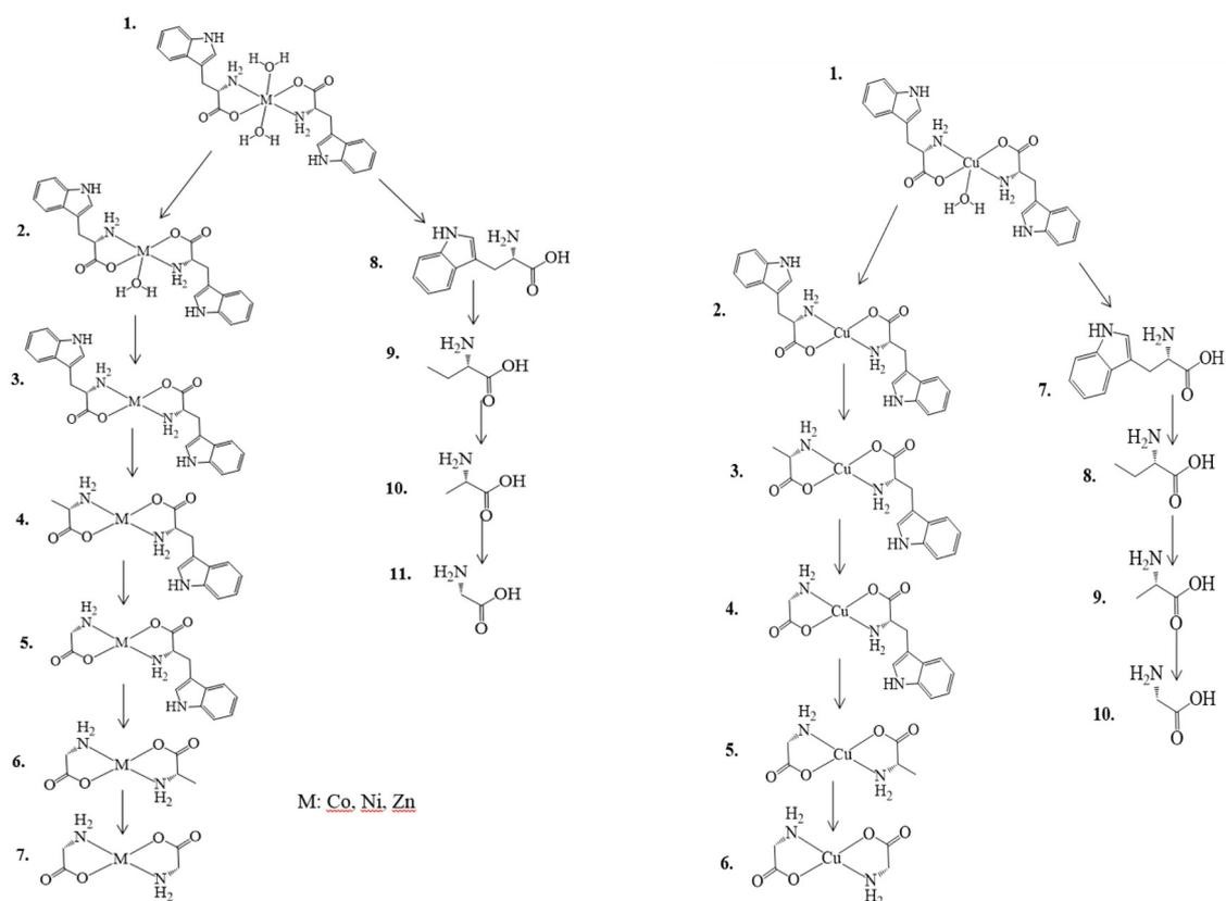
**Scheme 1.** Mass spectral fragmentation pattern of the metal complexes. (a) Co<sup>II</sup>, Ni<sup>II</sup> and Zn<sup>II</sup>; (b) Cu<sup>II</sup> complexes.
