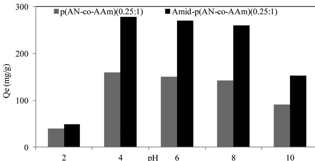
**Figure 6.** The effect of pH (2-10) on the sorption of  $\text{UO}_2^{2+}$  into p(AN-co-AAm) (0.25:1) and amid-p(AN-co-AAm)(0.25:1) [ $\text{UO}_2^{2+}$  concentration: 50mL,  $100 \text{ mgL}^{-1}$  adsorbent dosage :0.05 g].
