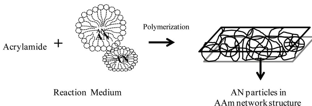
**Figure 1.** The schematic representation of p(AN-co-AAm) hydrogel synthesis.
