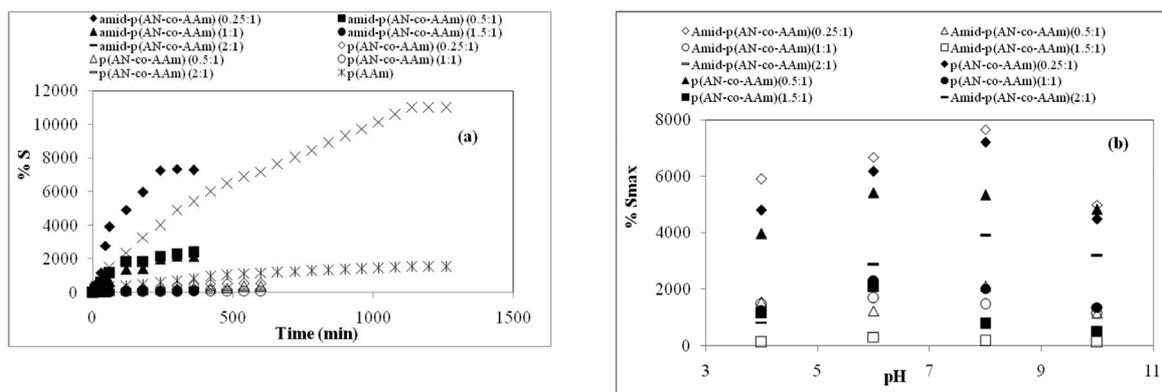
**Figure 2.** (a) Percent swelling degrees of hydrogels with time in DI water (% S vs time), and (b) Swelling of hydrogels as a functional of pH.
