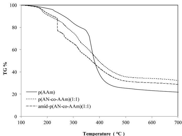
**Figure 4.** Thermogravimetric analysis of p(AAm), p(AN-co-AAm) (1:1), amid-p(AN-co-AAm) (1:1).
