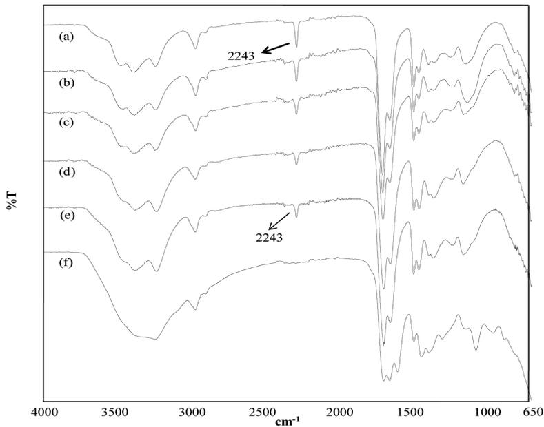
**Figure 3.** FT-IR analysis of (a) p(AN-co-AAm)(0.25:1), (b) p(AN-co-AAm)(0.5:1), (c) p(AN-co-AAm) (1:1), (d) p(AN-co-AAm)(1.5:1), (e) p(AN-co-AAm)(2:1) (f) p(AN-co-AAm) (2:1) after the amidoximation reaction.
