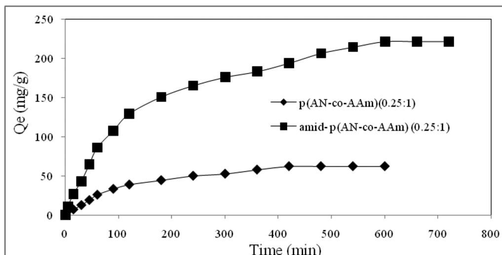
**Figure 5.** The amounts of absorbed  $UO_2^{2+}$  with time by p(AN-co-AAm) (0.25:1) and amid-p(AN-co-AAm) (0.25:1) hydrogels. [ $UO_2^{2+}$  concentration; 50 mL, 100 mg L<sup>-1</sup>, and adsorbent dosage :0.05 g].
