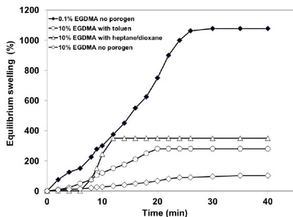
**Figure 9.** Equilibrium swelling of porous and non-porous PiBMA spheres crosslinking in gasoline.
