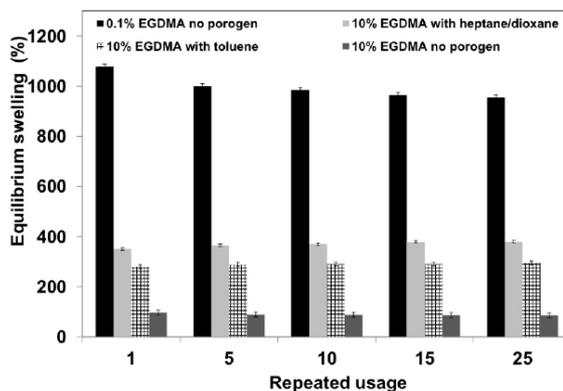
**Figure 10.** Equilibrium swelling with repeated usage, samples were swollen in gasoline and dried at in air at room temperature then in vacuum oven before tested each time.
