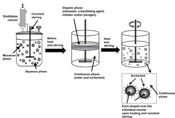
**Figure 1.** Suspension polymerization.
