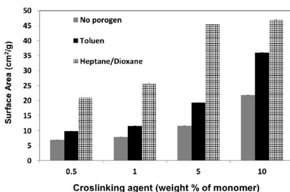
**Figure 7.** Surface area of porous and non-porous PIBMA spheres with respect to crosslinking agent prepared with 100% Toluene and 100%Heptane/dioxane (percentages are by volume of monomer phase).
