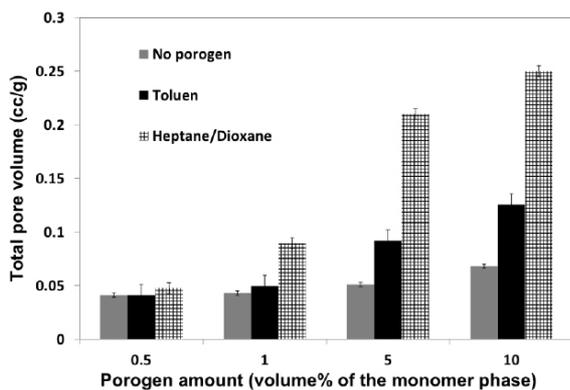
**Figure 5.** Total pore volume of porous and non-porous PIBMA spheres with respect to crosslinking agent prepared with 100% Toluene and 100%Heptane/dioxane (percentages are by volume of monomer phase).
