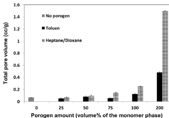
**Figure 6.** Total pore volume of porous and non-porous PIBMA spheres with varying porogen amount by volume of monomer phase (all samples were crosslinked with 10%EGDMA).
