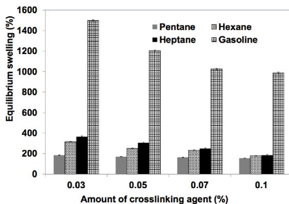
**Figure 2.** Equilibrium swelling of non-porous PiBMA spheres crosslinking with EGDMA.
