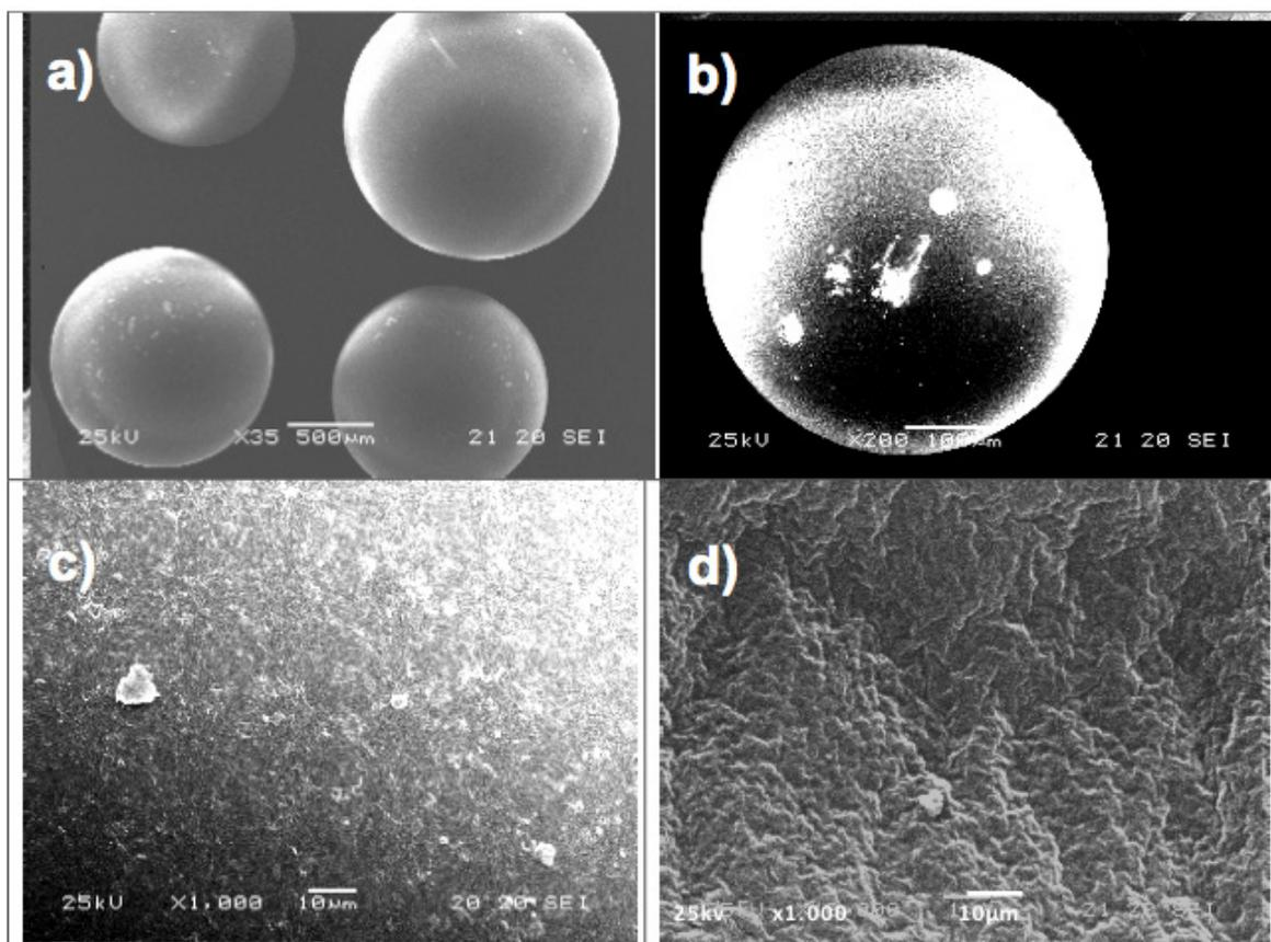
**Figure 4.** SEM pictures of a, c) non-porous b,d) porous PIBMA spheres prepared with 10%EGDMA and 100%toluene.
