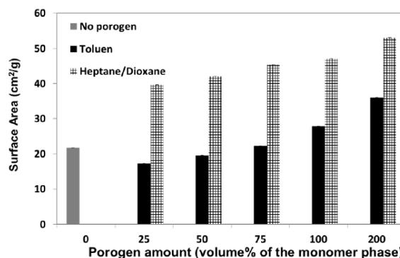
**Figure 8.** Surface area of porous and non-porous PIBMA spheres with varying porogen amount by volume of monomer phase (all samples were crosslinked with 10%EGDMA).
