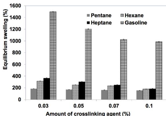
**Figure 3.** Equilibrium swelling of non-porous PIBMA spheres crosslinking with BDDMA.
